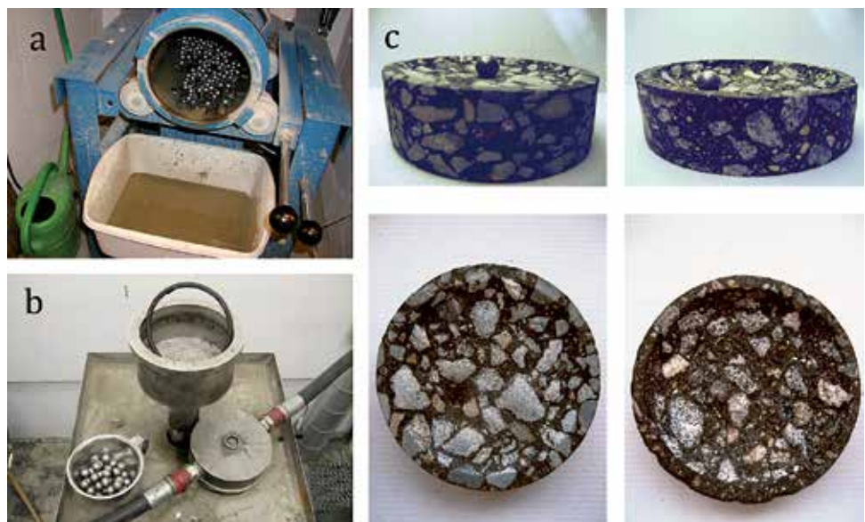
Figure 6: (a) Nordic Ball mill abrasion tester, (b) Prall tester, (c) asphalt mixtures tested by Prall.
