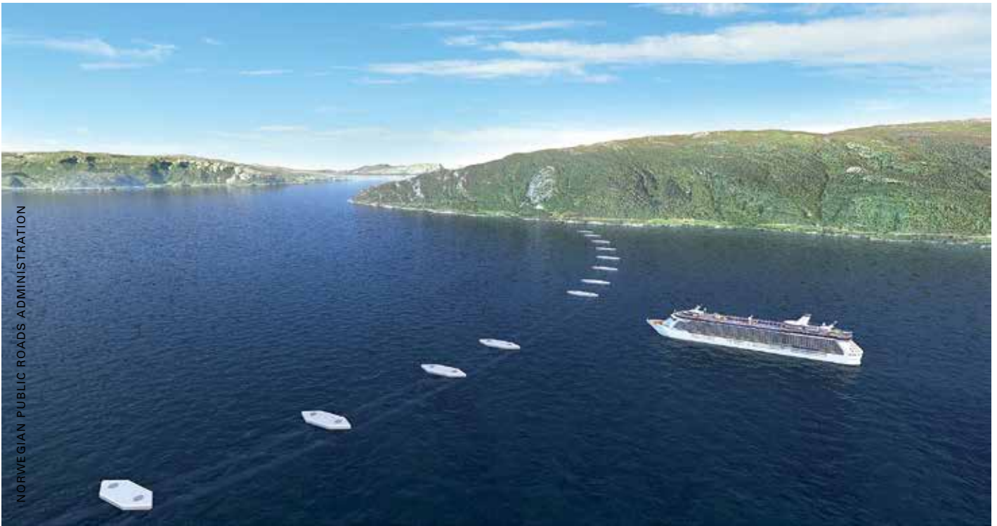
Floating tunnel held by floating pontoons.
