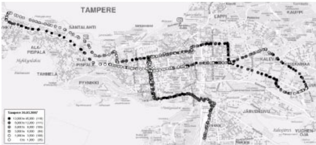
Figure 1. Respirable road dust on the streets of Tampere in 26.3.2007 in \mu\text{g}/\text{m}^3 (micrograms per cubic meter). The streets in the city center had relatively low emissions (pale circles) the "hot spot" streets with high emissions are plotted dark.
